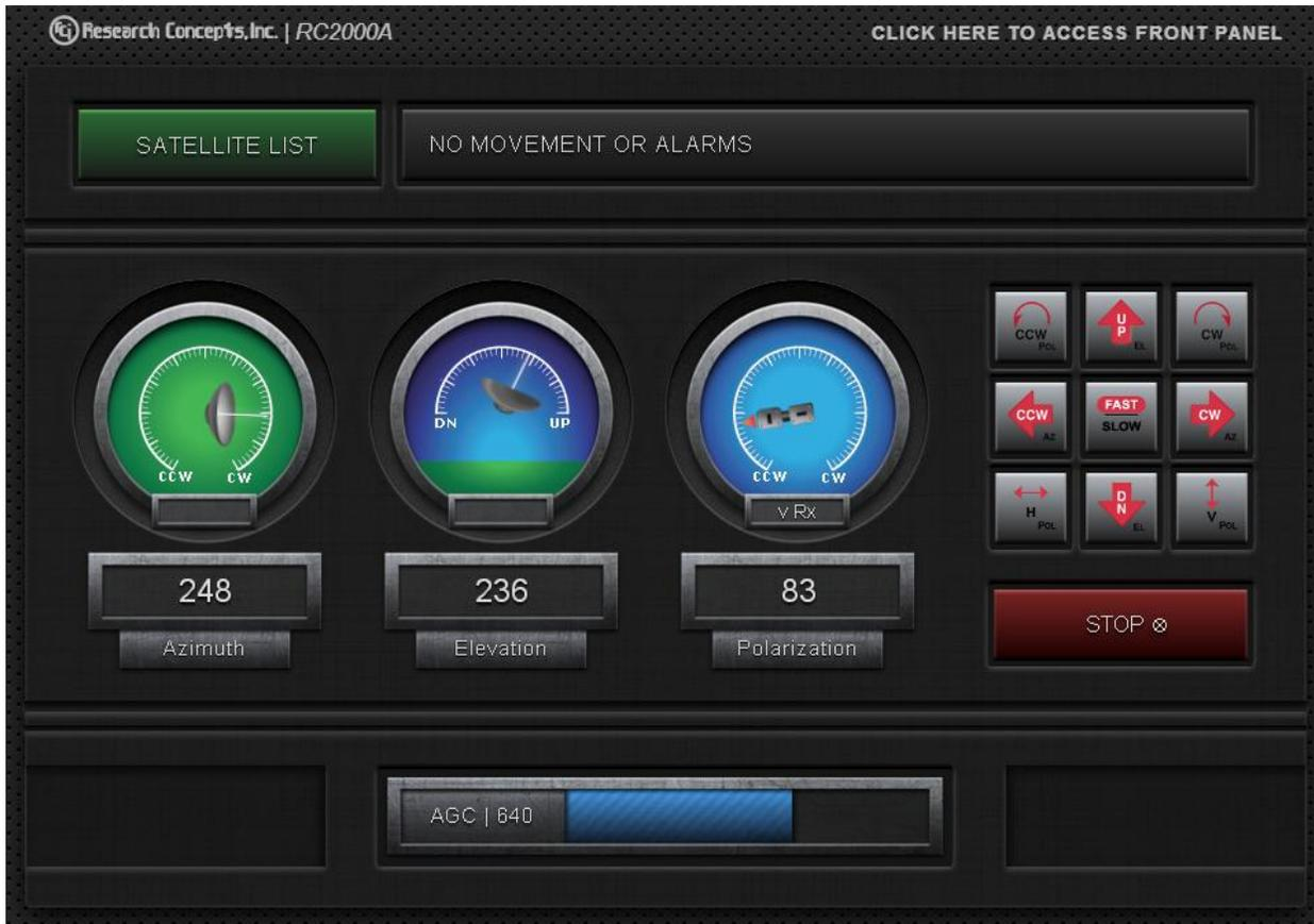
The RC2000A (version 2.70 and up) and the RC2000X (version 1.70 and up) can also access the Remote Front Panel. Pressing keys on the panel performs the same action as if keys were actually pressed on the front panel.
