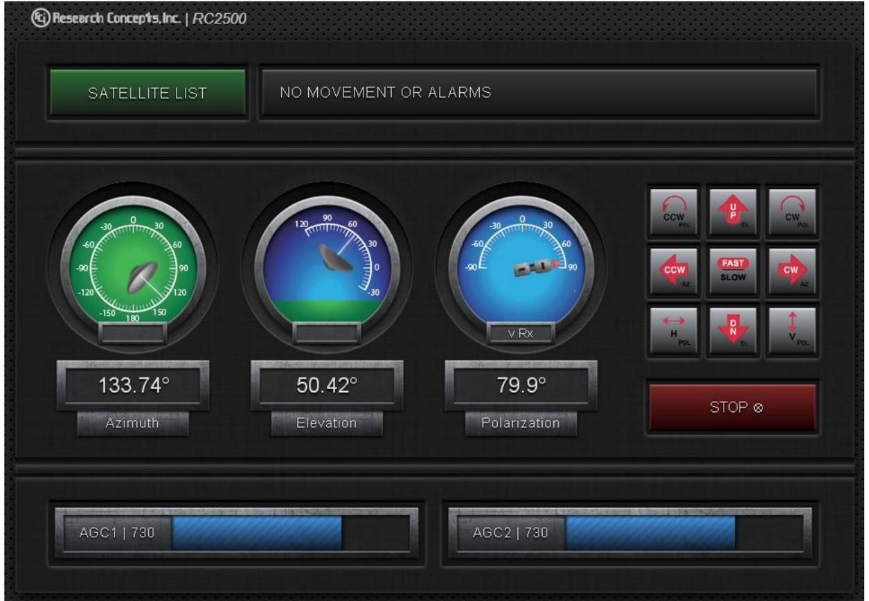
The RC2000A, RC2000C and RC2000X User Interfaces contain three gauges for displaying Azimuth, Elevation and Polarization position, a jog panel, two AGC outputs as well as a Satellite List. The Satellite list is automatically populated using the data previously setup in the RC2000. Selecting a satellite name from the Satellite List will begin an Auto Move to that saved satellite.
