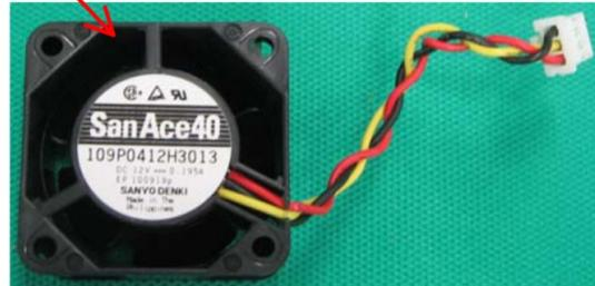
Step 4: Connect the fan cable with new fan to the Unit.
