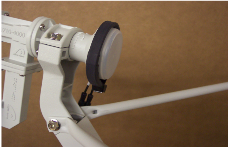
Feedhorn Heater Placement
