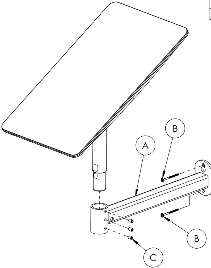
ATTACH THE LWM ARM TO A SUITABLE STRUCTURE WITH TWO RSS LAG SCREWS . MOUNT SHOULD BE LEVEL/PLUMB. SILICONE IS PROVIDED TO SEAL LAG SCREW PENETRATIONS FROM MOISTURE AS NEEDED.
