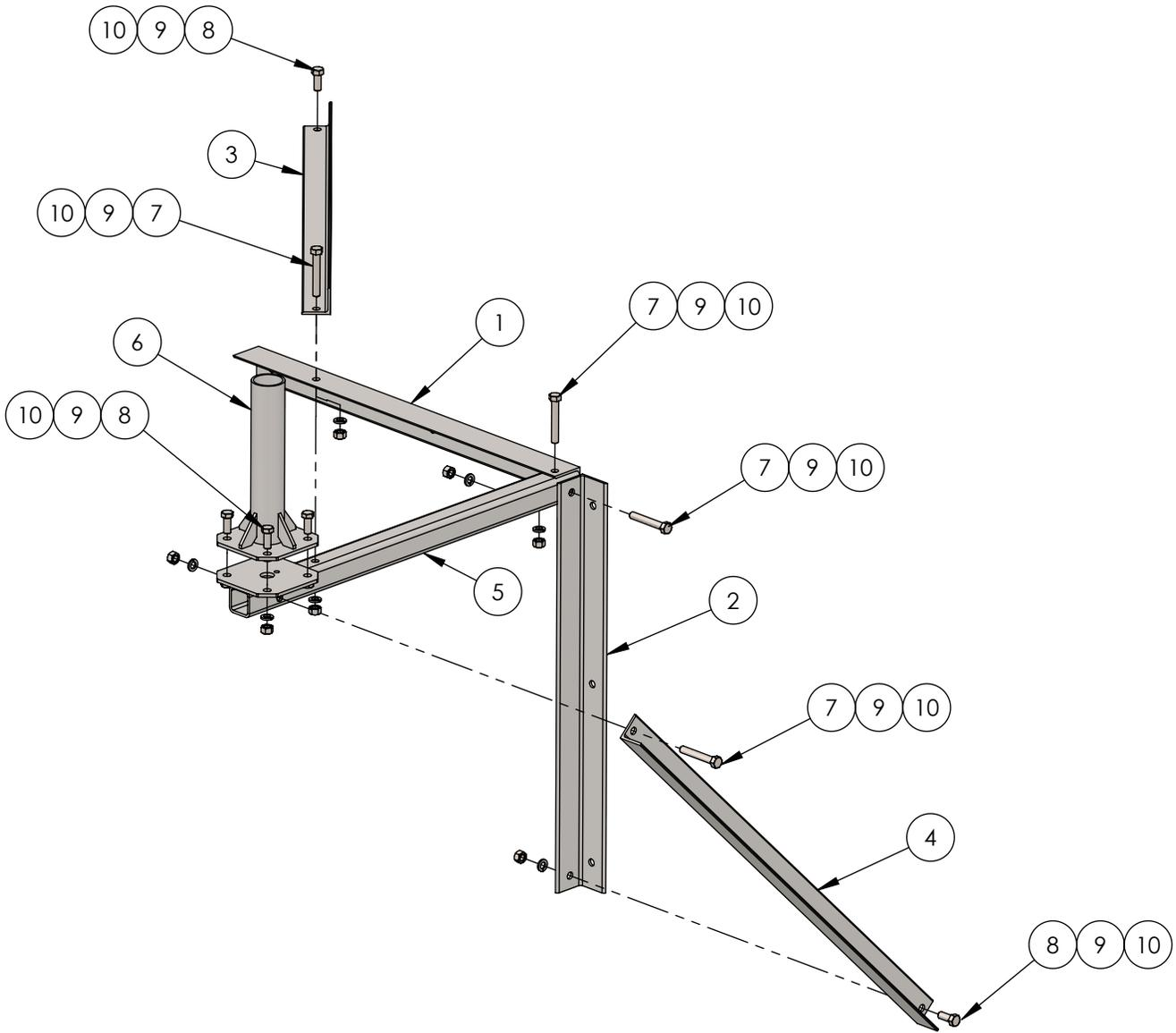
THE WL-4 CAN BE ASSEMBLDE IN AN LH OR RH VERSION (LH SHOWN ABOVE)
