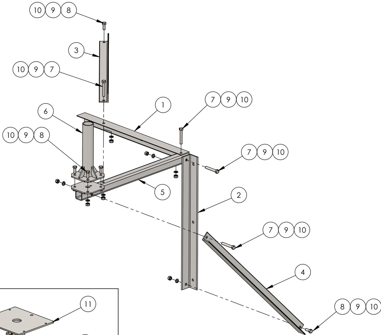
THE WL-4 CAN BE ASSEMBLED IN AN LH OR RH VERSION (LH SHOWN ABOVE)
