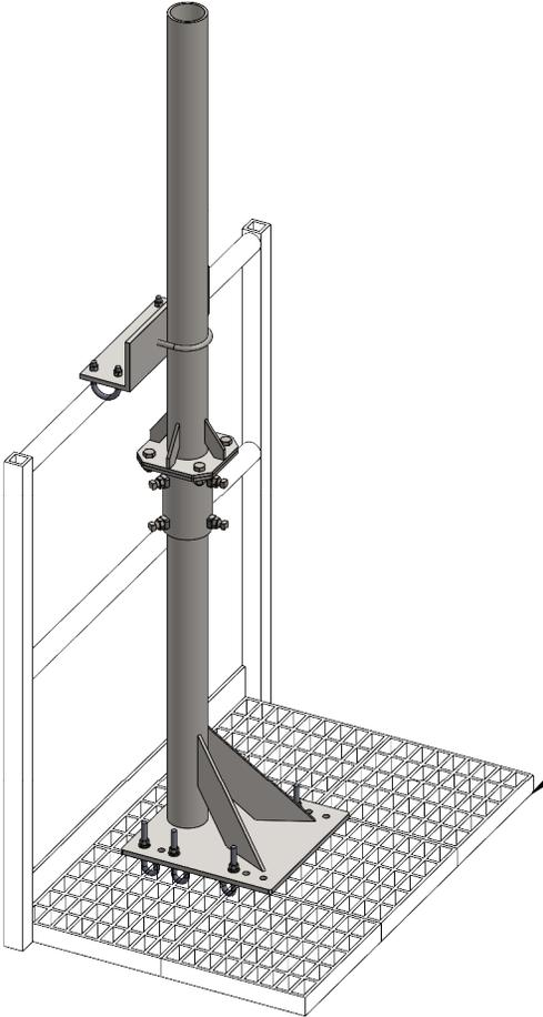
PARTIAL PLATROFM AND HANDRAIL SHOWN FOR EXAMPLE ONLY AND IS NOT PART OF THE MOUNT.
