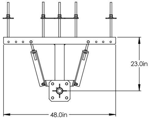
MOUNT IS SHOWN WITH THE THRU-WALL MOUNTING KIT COMES STANDARD WITH THE WL2-23 WALL MOUNT.
