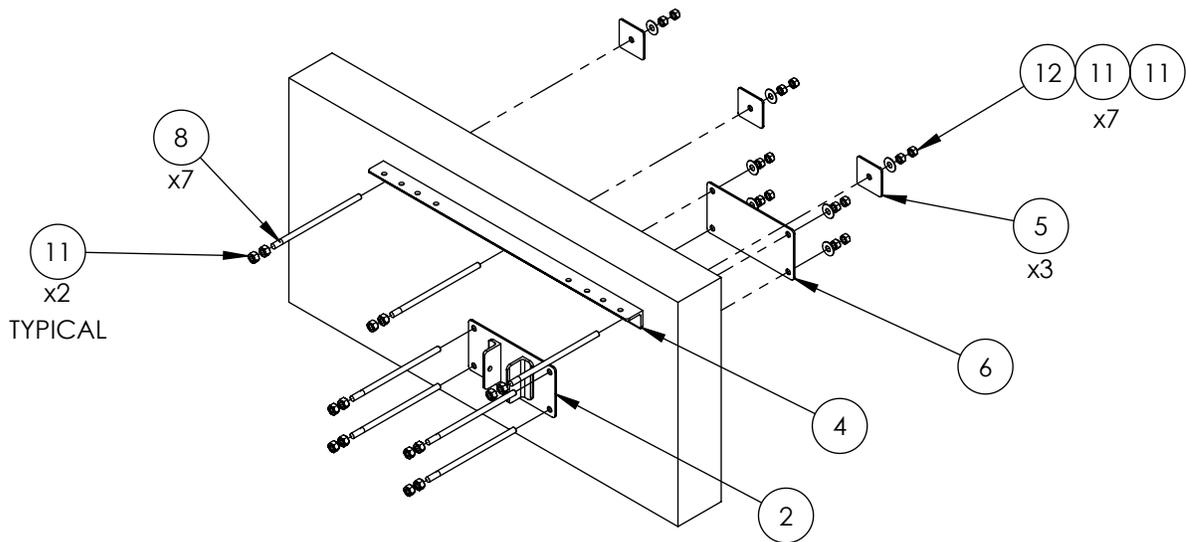
ATTACH THE UPPER WALL ANGLE AND THE LOWER BASE ASSY TO THE WALL(SEE DIAGRAM ABOVE)
