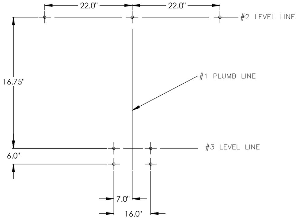
LAYOUT THE MOUNTING HOLE PATTERN AS SHOWN ABOVE. HOLES SIZED FOR 3/4" DIAMETER HARDWARE.
