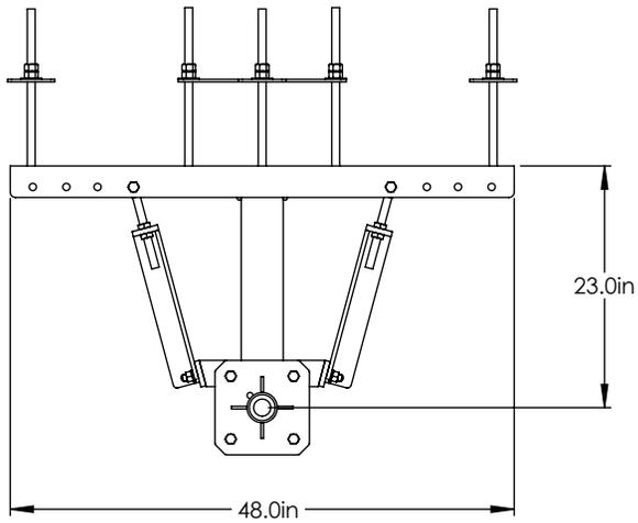
**MOUNT IS SHOWN WITH THE THRU-WALL MOUNTING KIT COMES STANDARD WITH THE WL2-23 WALL MOUNT.**
