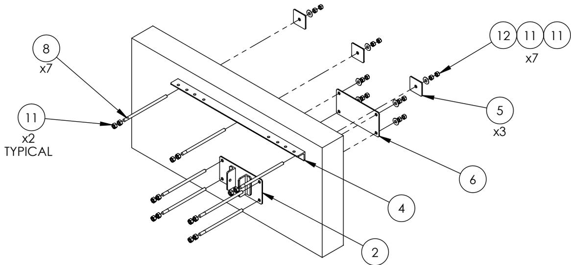
ATTACH THE UPPER WALL ANGLE AND THE LOWER BASE ASSY TO THE WALL(SEE DIAGRAM ABOVE)
