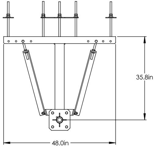
MOUNT IS SHOWN WITH THE THRU-WALL MOUNTING KIT. COMES STANDARD WITH THE WL2-36 WALL MOUNT.
