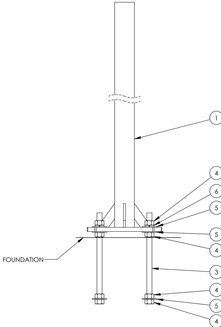
Remove the wood template after the concrete has cured. Clean the exposed threads and turn a nut all the way down to the top of the concrete on each rod. Set the pedestal and tighten hardware. See the drawing above.
