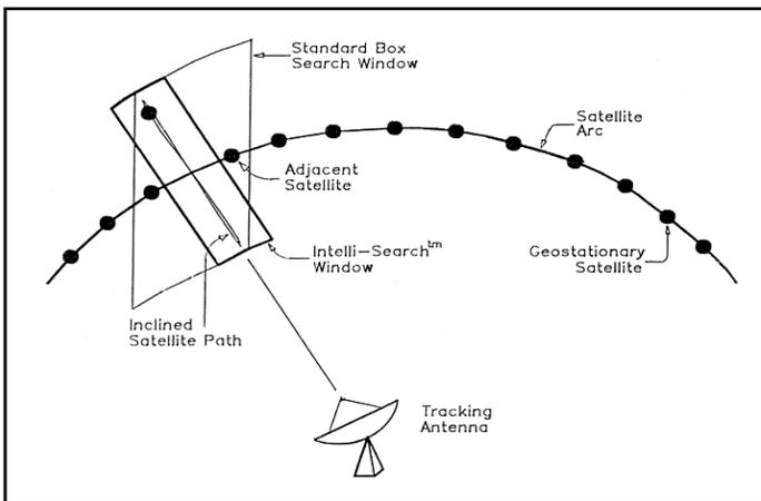
coincides with the satellite's expected path. Once an inclined satellite has been stored in the RC2000C, finding it again is as easy as locating a fixed satellite. Simply move to Auto mode, select the satellite from the list of those available, specify the proper polarization, and let the RC2000C do the rest.
