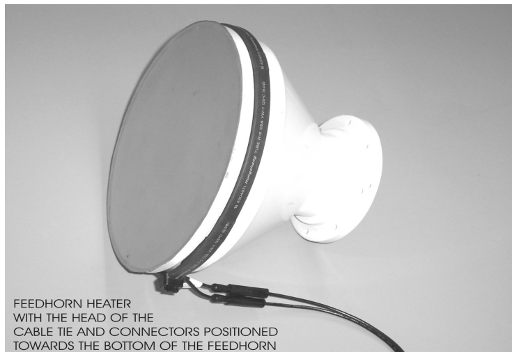
Feedhorn Heater Placement
