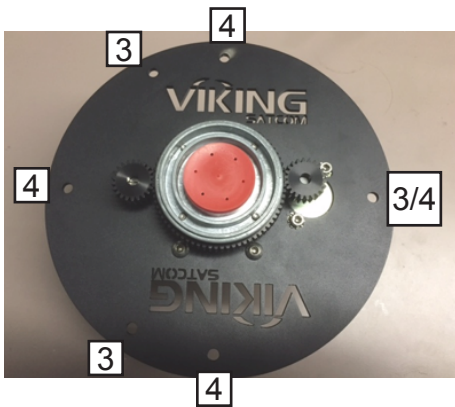
Three and Four Hole Bolt Pattern Used for Tri/Quad Strut Mounting
