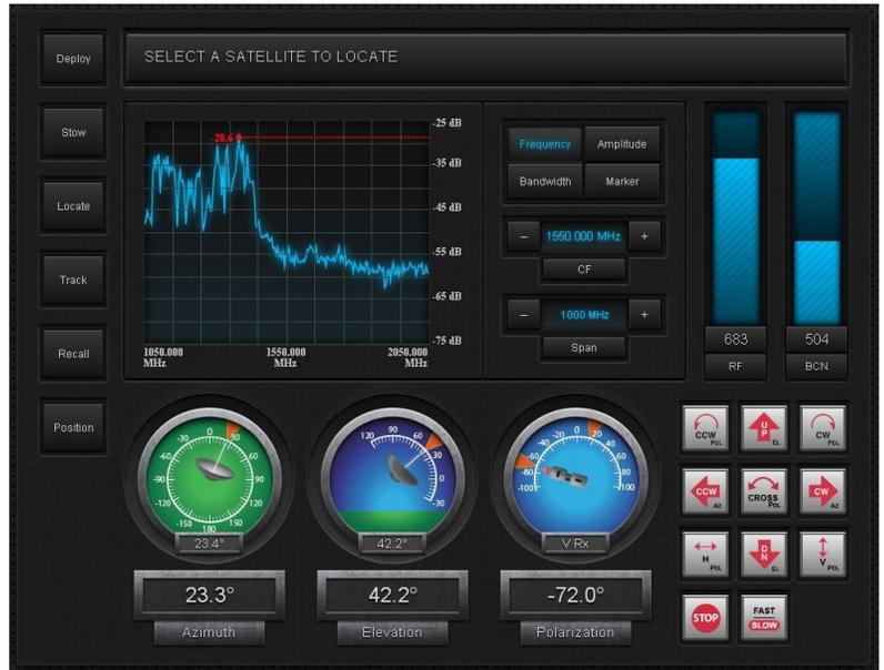
The RC4500-7200 Antenna Controller is a direct replacement for the Vertex/GD 7200 ACU. The RC4500-7200 can interface directly to a 7150 outdoor box, or can be used with an RCI designed outdoor unit.
